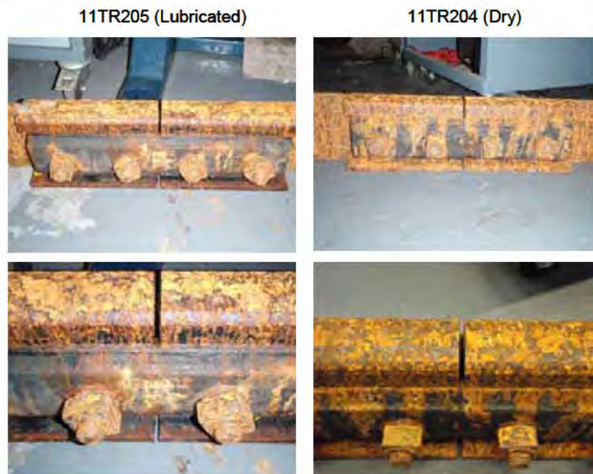
Figure 4: The two fishplate joints after corrosion for 150 hours
