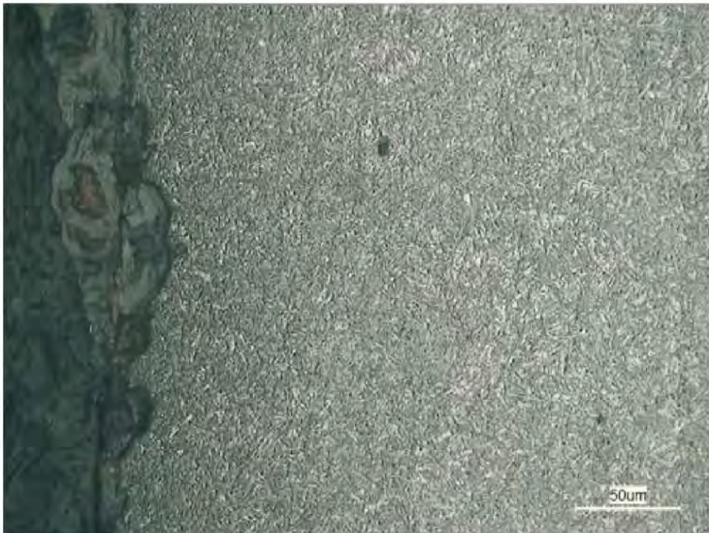
Figure 3.8. Image detailing bolt surface behind the fracture. Note the presence of pitting.
