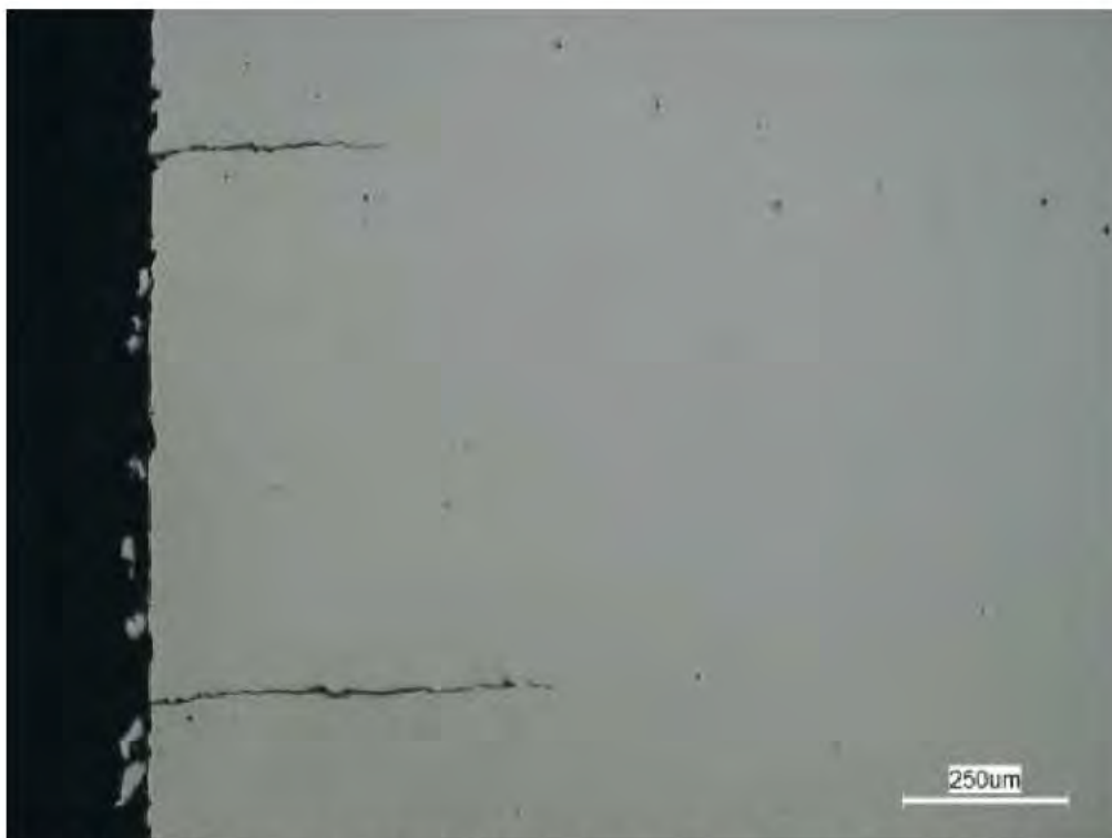
Figure 3.4. Image detailing bolt surface behind the fracture. Note the presence of multiple cracks.
