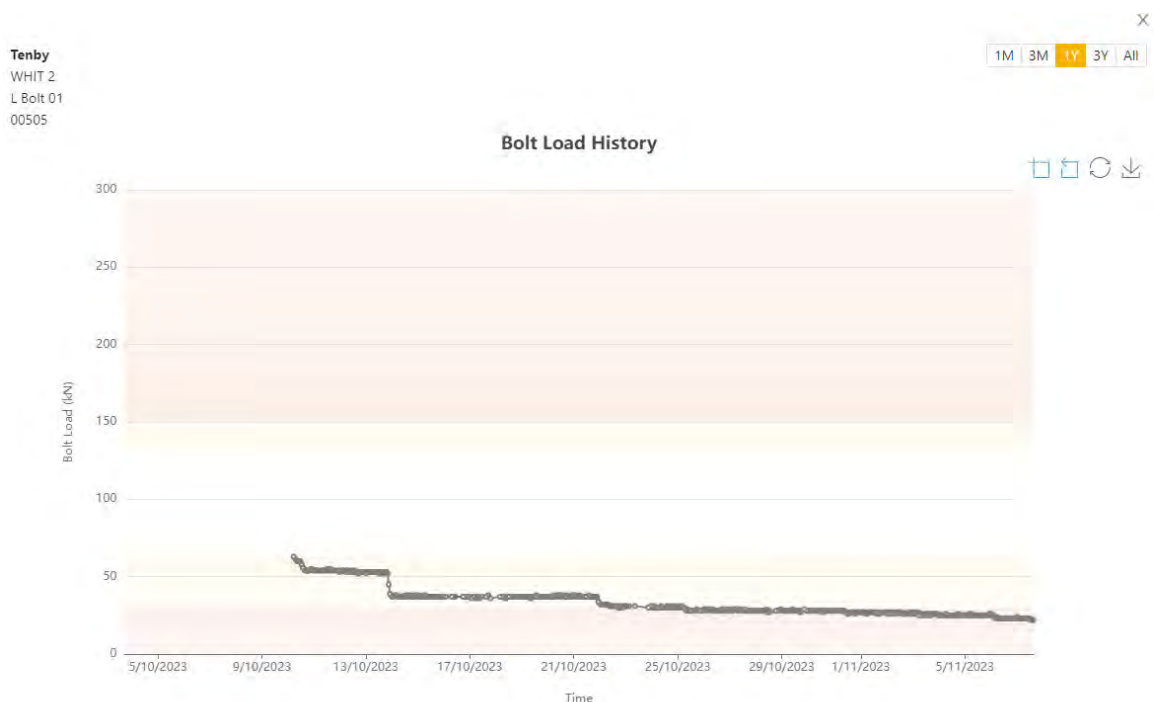
Figure 7. Bolt load over time for metric bolt 00505.
