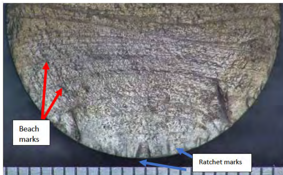
Figure 2.5. Image detailing fracture surface after cleaning. Note ratchet marks associated with larger fatigue crack located at the lower region of the fracture surface. Also note the presence of beach marks.
