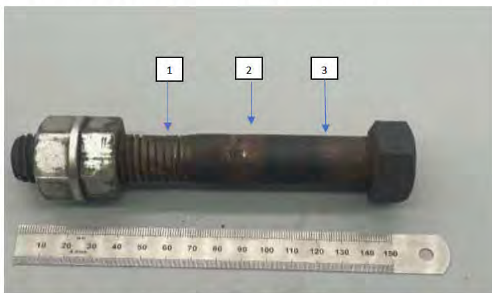
Figure 2.1. Image detailing fish bolt: note damage to threads.
