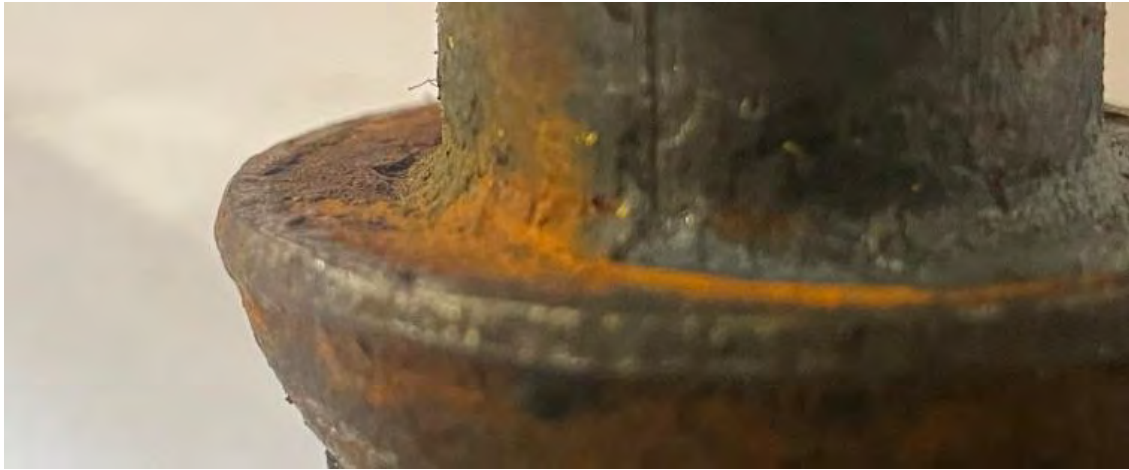
Figure 1. Underhead condition of imperial bolt.
