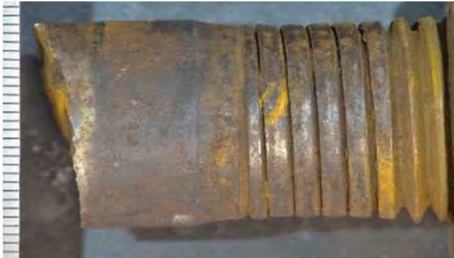
Figure 2.2. Image side 2 of bolt: Not damage to threads where the bolt was fixed through a fish plate. Note also an orange/brown deposit.
