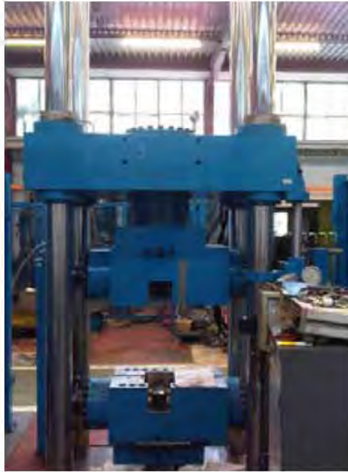
Figure 2: Servo hydraulic test rig – overall view (left) and with test specimen (right)
