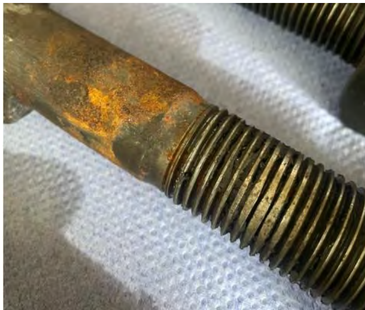
Figure 5. Damaged threads on imperial bolt.
