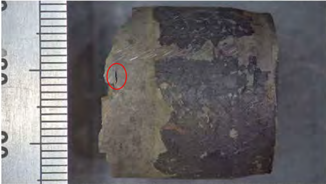
Figure 2.8. Image detailing surface adjacent to fracture, after cleaning. Note the presence of a small secondary crack (red circle).
