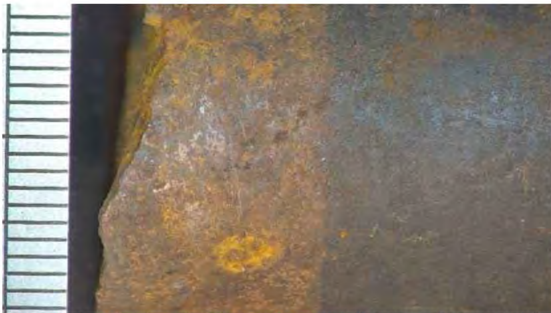
Figure 2.7. Image detailing surface adjacent to fracture. Note the presence of pitting associated with a corrosion deposit.
