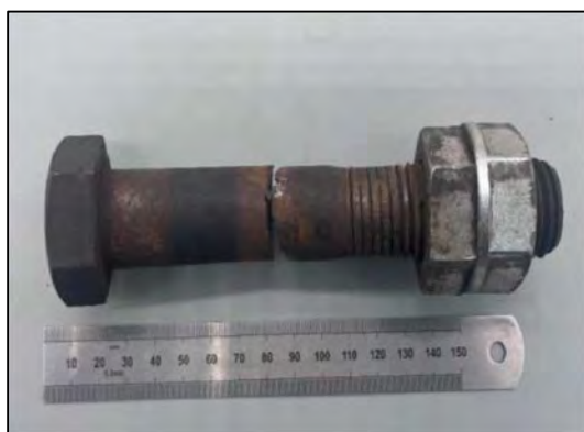
Failed metric bolt due to corrosion
