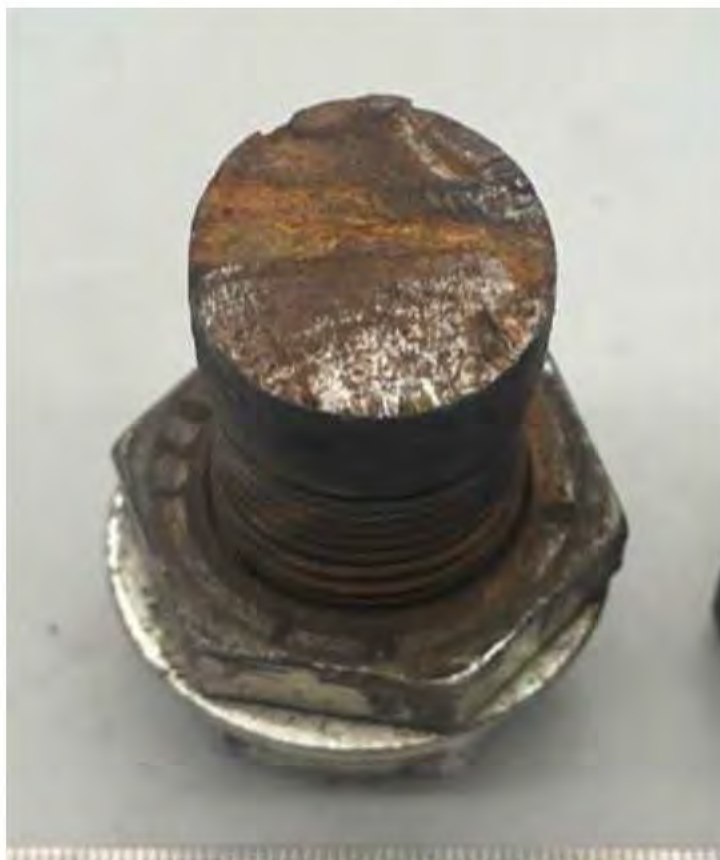
Figure 2.3. Image detailing fracture surface of side 2. Note the presence of an orange/brown coloured deposit across the surface.
