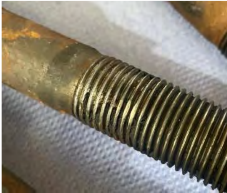
Figure 6. Damaged threads on imperial bolt.
