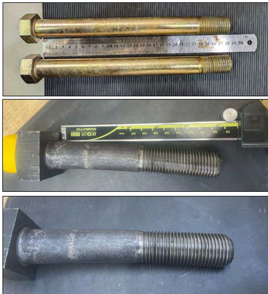
Images show failed bolts under load test.
