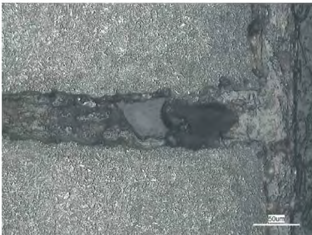
Figure 3.6. Image detailing bolt surface behind the fracture. Note the presence of corrosion deposit within the “spear-like” crack.
