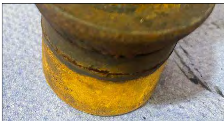
Bolt corrosion leading to seal failure and moisture ingress
